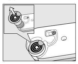
■ Remove the spout by holding the side lug and pulling upwards.
